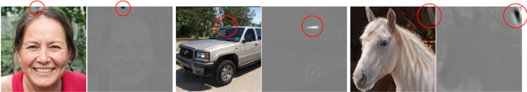
Figure 1. Instance normalization causes water droplet -like artifacts in StyleGAN images. These are not always obvious in the generated images, but if we look at the activations inside the generator network, the problem is always there, in all feature maps starting from the 64 \times 64 resolution. It is a systemic problem that plagues all StyleGAN images.
