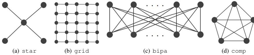
Fig. 2. Interference graph topologies: basic topologies
