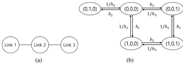
Fig. 1. (a) 3-link interference graph, where links 1 and 3 do not interfere with each other, but interfere only with link 2. (b) The resulting CSMA Markov chain for fixed parameters  $(b_1, b_2, b_3)$  and  $(h_1, h_2, h_3)$ , where for example the state  $(1, 0, 1)$  means that links 1 and 3 are active and link 2 is inactive.
