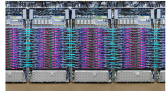
Cloud TPU v3 Pod 100+ petaflops 32 TB HBM 2-D toroidal mesh network
